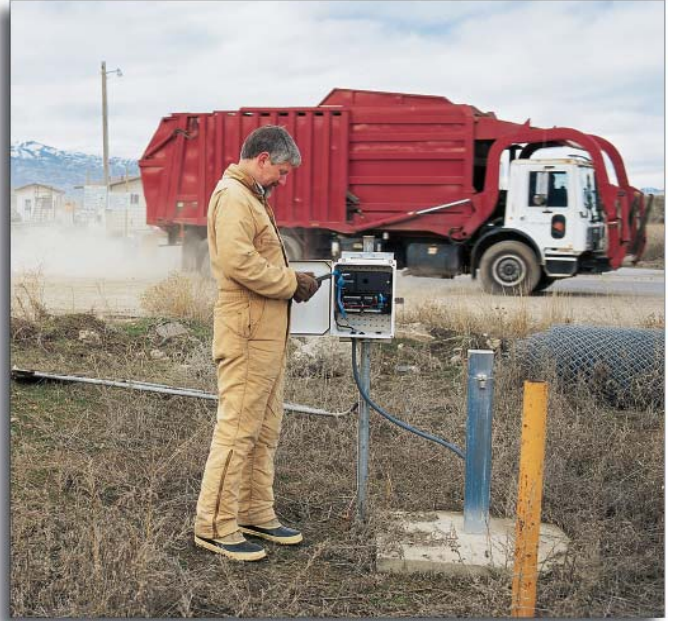
Our dataloggers are typically interrogated via telecommunications from an office, but you can also access the data on-site.
