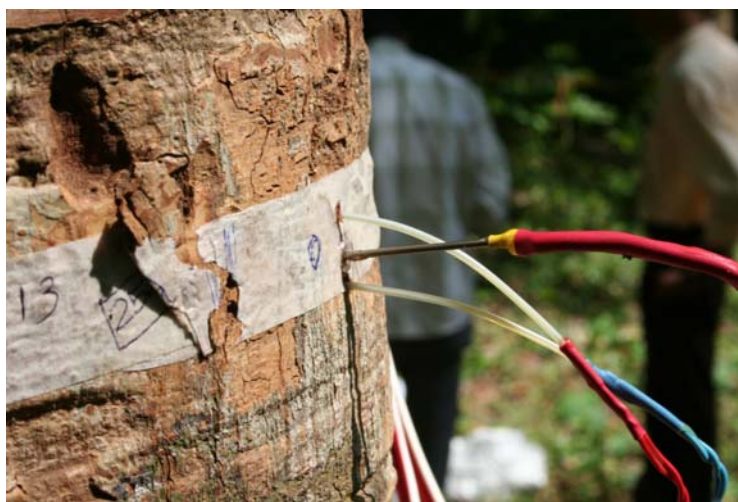
Tree trunk with the heater and temperature sensors inserted into the sapwood.
